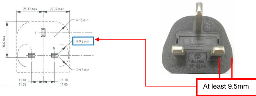
Figure 3: Distance of live/neutral pin to plug periphery for plugs manufactured by Ching Cheng Wire Material
